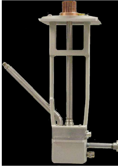
Figure 2. Model 74035 single-stage variable temperature oven
