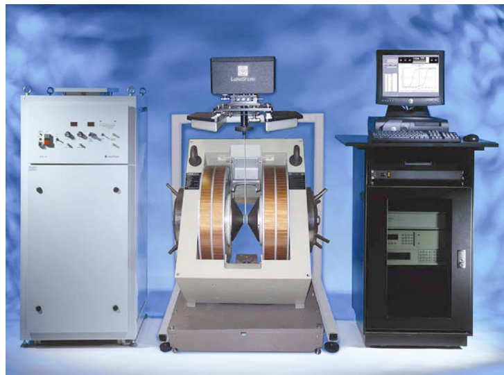
Figure 1. Lakeshore 7410 Vibrating Sample Magnetometer
