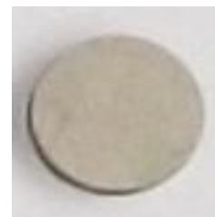
Figure 5. NiTi shape memory alloy can be sintered between 700 °C to 900 °C with 50 MPa pressure by SPS in two minutes
