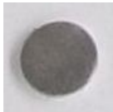
Figure 2. Tungsten carbide (WC) pellet sintered at 1800 °C with 50 MPa pressure using SPS
