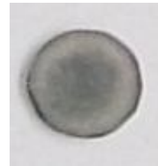
Figure 3. Silicon Nitride (Si 3 N 4 ) pellet prepared at 1600 °C with 20 MPa pressure using SPS
