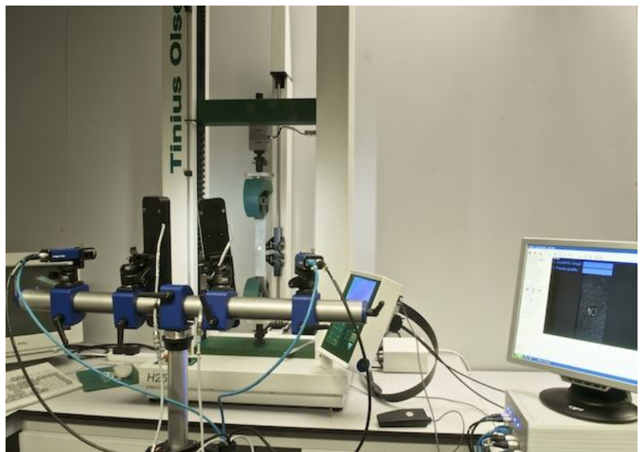
Figure 1. 3D Digital Image Correlation (DIC) system analysing glass-fibre reinforced composite single-lap, single-bolt bolted joint.
