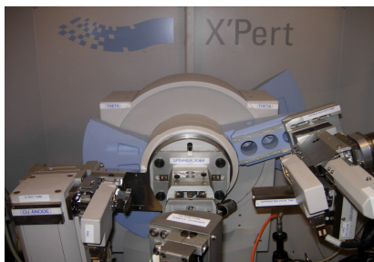
Figure 1. Phase analysis on powder even on very small sample quantities
