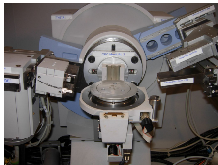
Figure 2 Thin film, glancing angle... modules for different applications.
