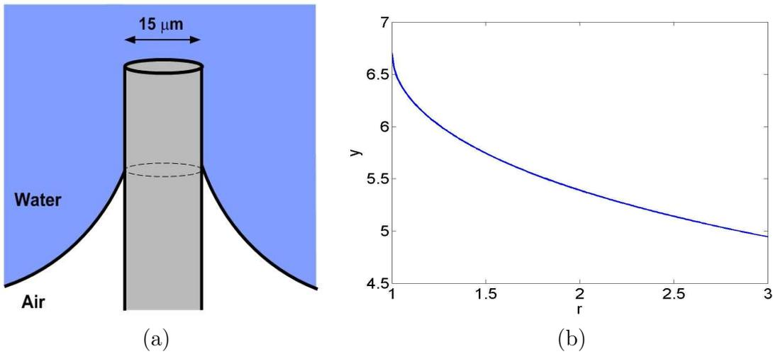
Figure 7: (a) Schematic of liquid meniscus. (b) Dimensionless plot of liquid height  $y$  against distance from cylinder centre,  $r$ . We multiply dimensionless quantities by  $R$  to convert to dimensional quantities. The contact angle was taken to be  $170^\circ$ .
