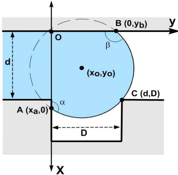
Figure 9: Schematic of liquid going through the microchannel.
