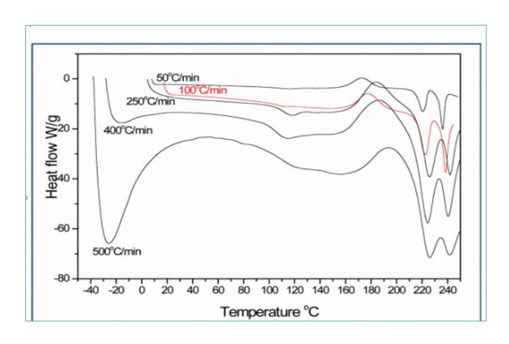
Different ramp rates can show how the sensitivity towards the thermal transitions of a sample is increased at high heating rates (endothermic peaks are down)
