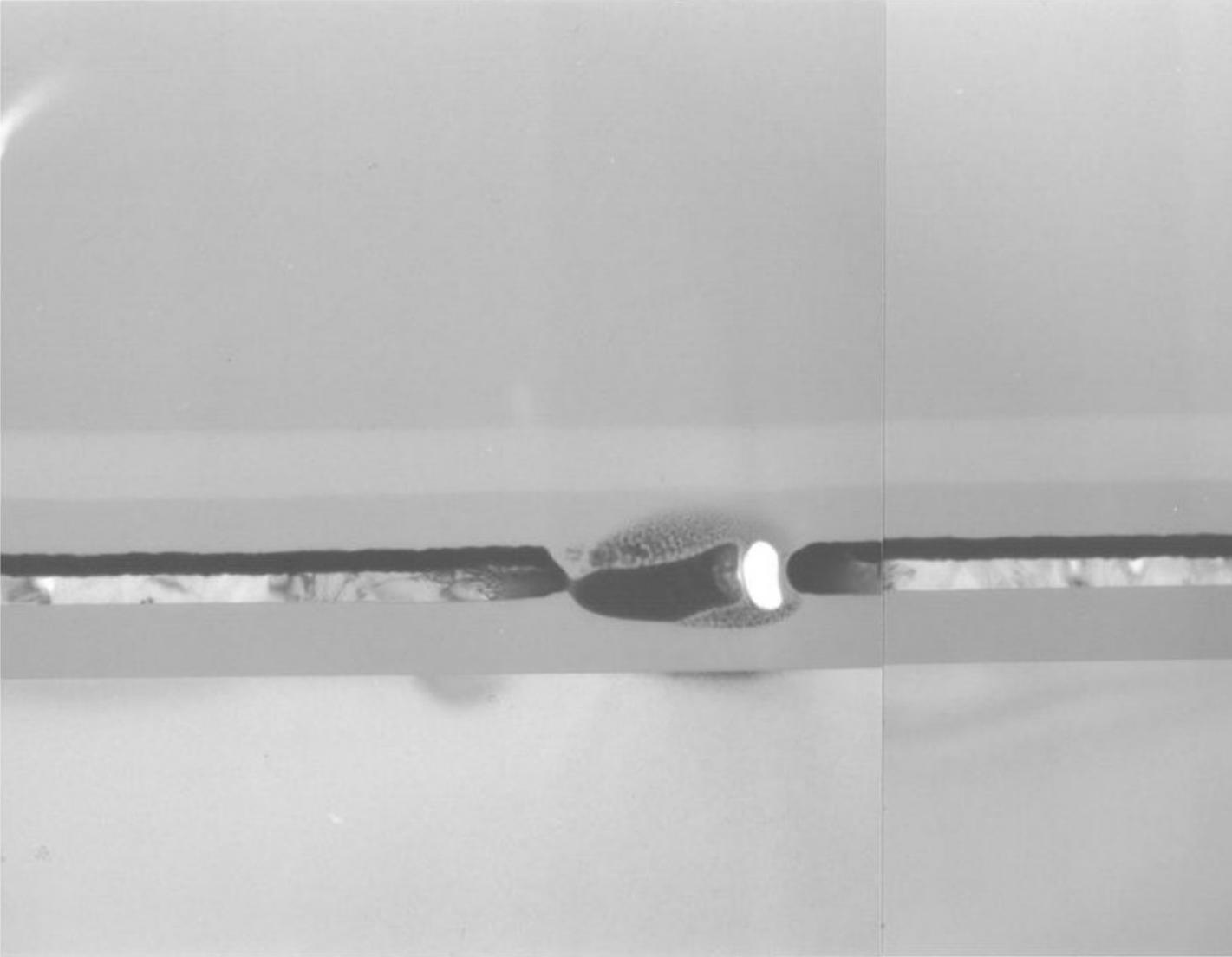
Figure 3: As figure 2. Side view showing the layer of tungsten silicide above (dark) and the polysilicide below to which the tungsten silicide is attached. Examples of necking (incomplete pinch-off?) at the left and the pinch-off by insulating material around the white cavity at the right, are clearly shown. [Courtesy *Analog Devices*.]
