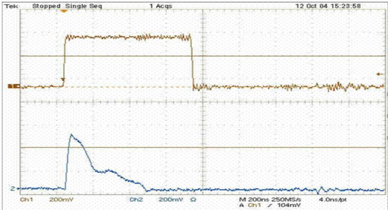
Figure 1: Upper plot: voltage across the fuse. Lower plot: the current  $I(t)$  through the fuse as a function of time  $t$  after the voltage is first applied across the fuse. The initial current rise, to a peak of about 90 milliamps, is in a time of 1 nanosecond or less (it is quicker than the instrument could measure). The width of the upper half of the peak in current is about 40 nanoseconds. The whole blowing process is completed in 500 nanoseconds. [Courtesy *Analog Devices*.]
